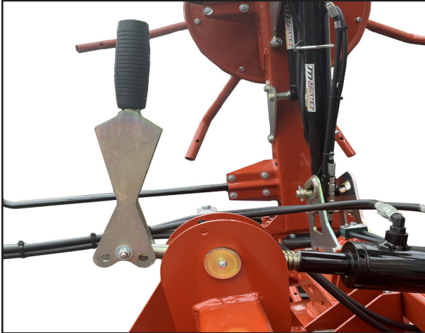
Figure 5: Tilt Cylinder adjustment Position
