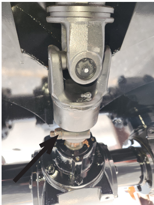
Figure 23: The rear PTO shaft should not be frequently removed. To secure the rear PTO tapered pin on the beater side connection, tighten the nut on the PTO connection to the 1-3/4" diameter 6 splined shaft to 162 ft. lb.
