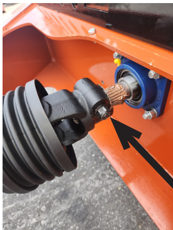
Figure 21: The front Power Take-Off (PTO) shaft should not be frequently removed. To secure the front PTO tapered pin, tighten the nut on the PTO connected to the 1-3/8" diameter 21 T splined shaft to 110 ft-lb of torque.
