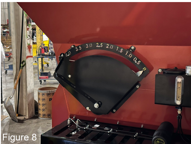
Figure 8: The arrow indicates the gate height measured in feet. The arrow indicates the distance from the bottom of the endgate to the floor. Regularly check that when the endgate is lowered, the indicator arrow reads zero, and when fully raised, it reads 4 feet.
