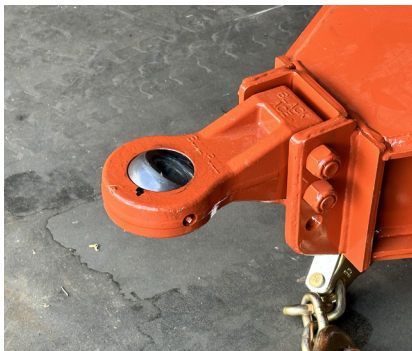
Figure 20: Bull Pull optional hitch shown to the left. Lubricate after every 40 hrs of use.
