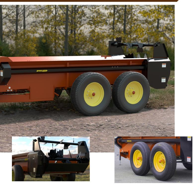
The optional fine spread pan, available on all models, prevents finer or dry manure from falling out of the box in transit and in the field.
