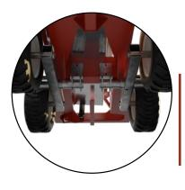
Extreme Duty Tandem Walking Beam is standard on all models. These heavy parts add to the stability to the unit during unit dumping
