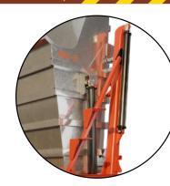
Standard double cylinder circuits gives better control during dumping.
