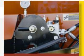
Floor control With standard reverse feature to easily clear out any plug ups Standard Web Bearing Timken double tapered roller bearing is standard for the extra heavy duty web chain
