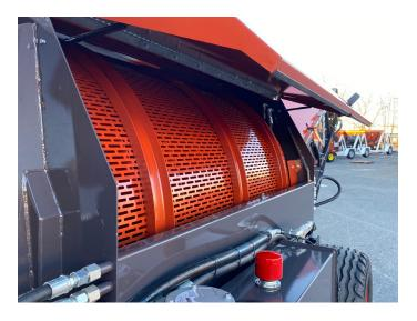
The patented cleaning drum removes most of the dust and small debris collected from the windrow. The auger flighting inside the drum forces the nuts to travel across over 60 feet of the cleaning slots. This process removes such a significant amount of debris that in many conditions the blower is not even used. This process virtually eliminates significant airborne dust.
