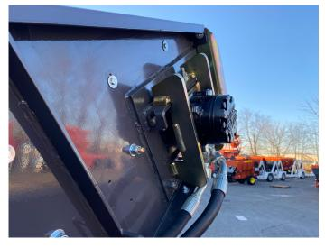
Exclusive low profile, direct drive motor eliminates the need for drive chain adjustment or replacement.
