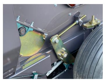
Heavy duty tensioner extends the life of the pick up chain and makes maintenance a breeze.
