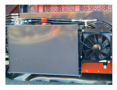
The oversized tank and the standard oil cooler ensure a low operating temperature of the hydraulic fluid.
