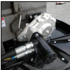
Rawson 6:1 Hydraulic Drive Gearbox
