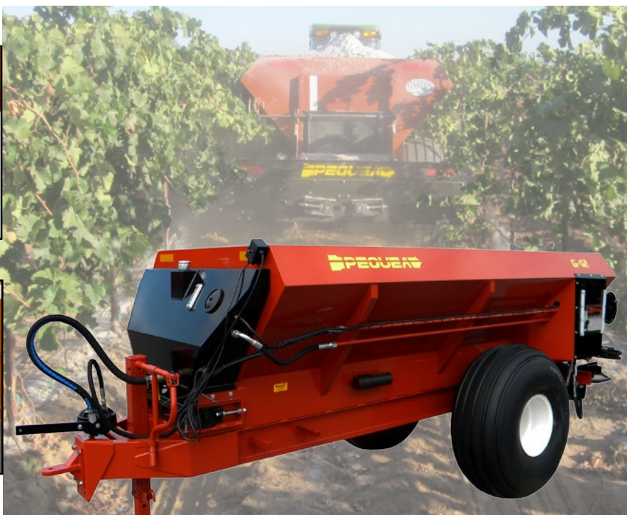
Adjustable Axle (Standard) 6" of Height Adjustment
