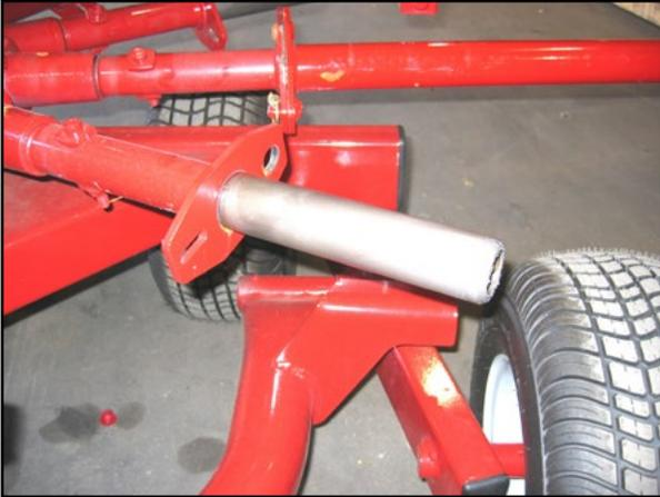
Remove rubber caps from gearbox stub shaft. Remove tine arms from storage position and slide onto gearbox stub shaft. Insert tab on tine arm into slot and insert locking pin. Rotate gearbox installing tine arms until complete. Do not operate without all arms installed correctly.
