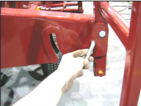
To lower the guards, simply pull the locking pin and slowly lower the guard to the raking position and reinsert pin to lock in place. Guards should also be stored in transport position.
