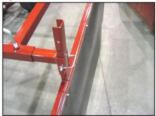
Slide curtain assembly into receivers on guard and insert locking pins at desired height. The locking bolts on the guard allow for quick horizontal adjustment in the field to adjust the width of the windrow.
