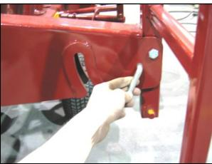
To lower the guards, simply pull the locking pin and slowly lower the guard to the raking position and reinsert pin to lock in place. Guards should also be stored in transport position.
