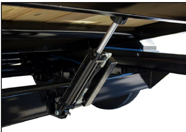
Hydraulic Cushioned Gravity Tilt (No Power Required)
