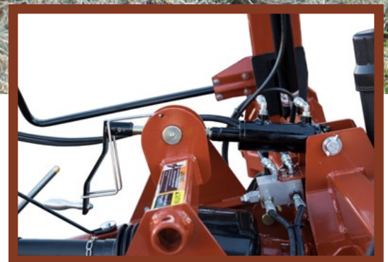
The HT4102 was designed to make maintenance easy - with the hydraulic manifold mounted right next to the front tilt cylinder, it makes it simple to check or tighten hoses.
