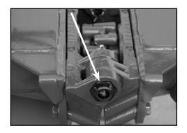
The tilt cylinder adjustment threads must be kept well greased to allow for easy adjustment for tine height.
