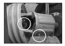
The radial pin clutch and the center cross in the pto yoke should be greased every 8 hours.
