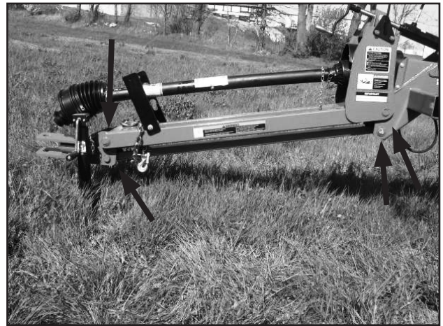
Tongue leveling pivots, 2 front, 2 rear
