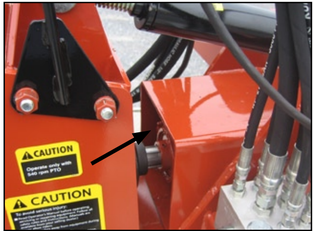
Flange bearing on drive shaft
