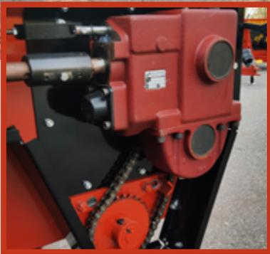
Our large PTO model manure spreaders include 2 speed gearboxes with a neutral and cleanout setting.
