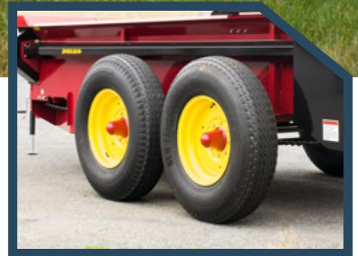
The tandem axle option provides better performance in harsh condition like rough terrain or wet fields.
