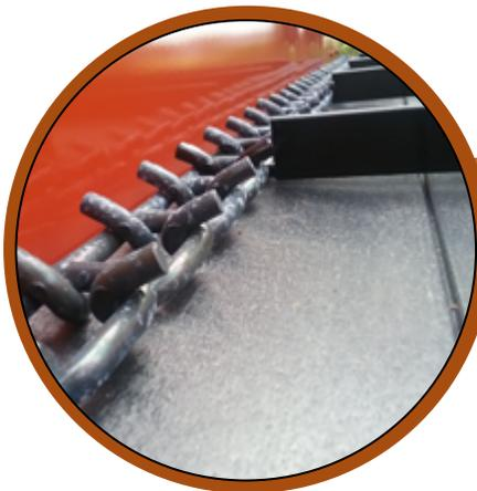
A Poly floor and T-rod chain makes these spreaders durable and long lasting
