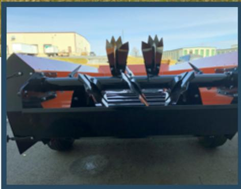
The optional fine spread pan, available on all models, prevents finer or dry manure from falling out of the box in transit and in the field.
