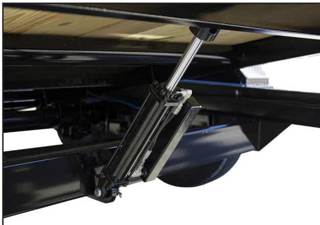
Hydraulic Cushioned Gravity Tilt (No Power Required)
