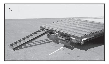
Check before each trip to insure that ramps are properly stowed and secured before moving trailer. Ladder ramps (1) may be secured in storage bins with a pin or on the rear of the trailer with straps. Straps may have a combination of bolts and nuts and/or pins to secure ramps in place.
