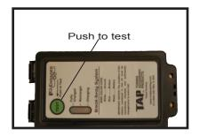
Check the breakaway system before each trip. If the battery is not fully charged, it should recharge automatically when the electrical system is connected to the tow vehicle. If any problems are encountered, consult your local dealer immediately.
