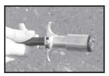
Check all wires and connections to ensure that they are in good condition and connections are secure. A short or break in the wiring can cause a failure in the breakaway function and result in damage to equipment, injury or death.
