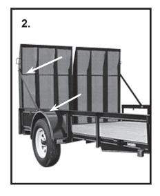
IMPORTANT: Always use stabilizer jacks when loading equipment heavier than the weight of the tow vehicle unless there are provisions for this built in to the ramps
