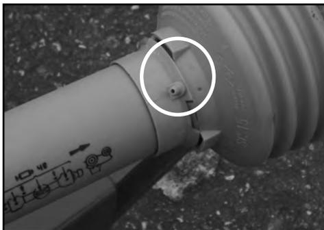
The pto guarding should be lubricated at all times. If the shield feels tight when it is extended and retracted then lubricate as necessary.
