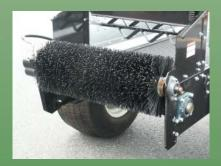
The optional brush allows for precise application of fine spread material.
